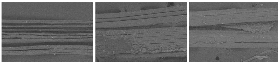
Fig. 1: SEM images (200X magnification) of flax fibres of Aretha Normandy (left), Aretha Melita (middle) and Aretha Portage (right).
